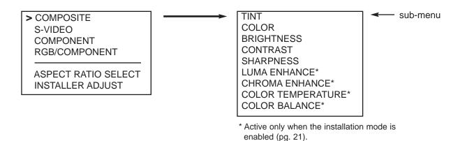
Picture quality adjustments (also known as "Front Panel Controls") are the controls that change different parameters of the image such as the amount of color, black level, etc. While these adjustments can be set to suit the needs of the user, there is a way to set these properly. This section will describe what each function does and how to adjust them properly.
